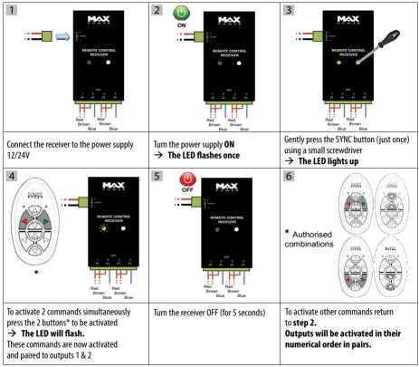
Note: Each receiver can handle a maximum of 4 channels: 2 sets of 2 buttons corresponding to receiver outputs (1, 2, 3 and 4). Should the full 8 channels of the transmitter be required, a second receiver is needed: 312971 (EU) or 312972 (US).
